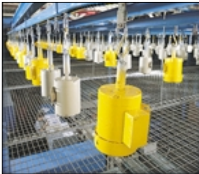
LEESON's flexible epoxy coating systems allow custom runs of WASHGUARD® and other severe-environment motors.
