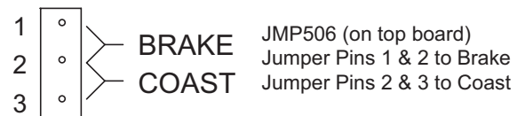
Figure 13. Jumper Settings--JMP506
