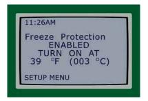
**WARNING:** Freeze Protection will ONLY function with the selector knob in the RUN position. Damage may occur to the user's pool system if Freeze Protection is enabled and the switch is not in the RUN position.
