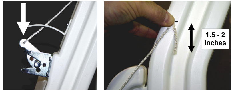
Step 4: Make sure gate latch catch is in down / locked position over striker bar. Extend string upwards to outside face of upper handrail & fold end approx. 1.5 - 2 inches. Mark handrail at fold in string for location of eye screw (see also Step 5 below)
