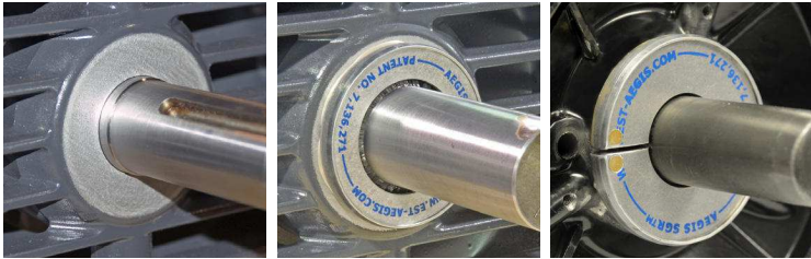
Cleaned shaft & end bracket Solid Ring Installed Split Ring Installed
