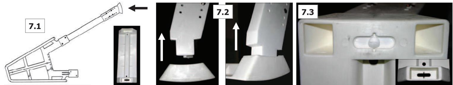
7. With the sub-assembled ladder on edge (7.1), fit a base tread D onto the C1 & C2 adjustable base supports (7.2). The base tread has a pocket at both ends that fits over the C1 & C2 base supports. The C1 & C2 base supports have a locking tab on the ends; press the base tread onto the base supports until the button-lock tab snaps through the bottom channels of the base tread (see 7.3). Position the locking tab in the center of the channel and snap firmly in place (7.4).
