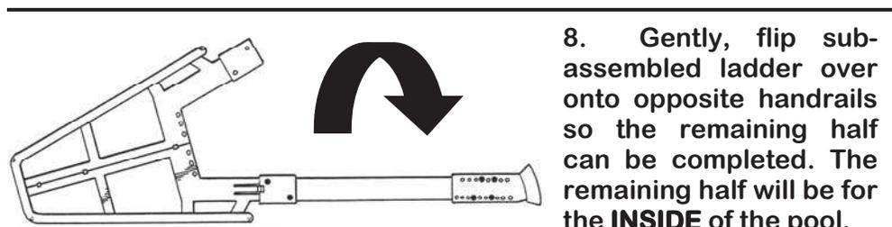
8. Gently, flip sub-assembled ladder over onto opposite handrails so the remaining half can be completed. The remaining half will be for the INSIDE of the pool.
