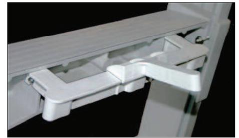
2. Fit sub-assembled BA+BC to back of in-pool ladder section F, behind top ladder tread/rung. The extended screw tabs on Part BC fit on the outside of the strengthening ribs of the tread/rung. Slide to top of ribs and secure in place using a 1/2" screw on both left & right sides.
