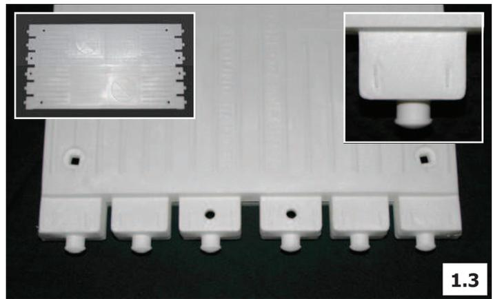
1. Position A1 & A2 handrail sets together as shown (1.1). Each handrail has holes to accept the top platform (1.2). The ends of the platform are designed to fit within these holes and snap & lock into place (1.3). Fit the platform, with anti-skid surface and warning labels facing upward, into the handrails (1.4). Gently tap outside of handrails so the button-lock tabs protrude through and secure platform in place. Make certain tabs lock securely (1.5). Repeat for both sets of handrails.
