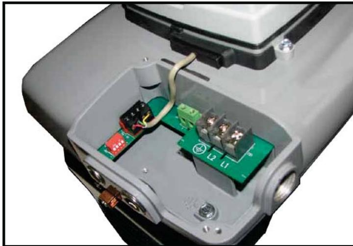
**Figure 12: Internal Plastic Cover Removed**
